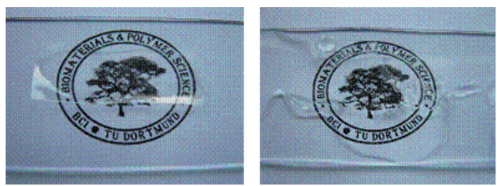
Figure 1: Photos of PHEA- l -PEtOx 4,8 conetwork in dried and water swollen state.
