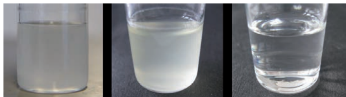
Figure 1: From left to right ~7 mg lysozyme in 5 ml DMF: native; modified with PADA (5.0 mg) only; modified with poly(2-methyl-1,3-oxazoline) (81.3 mg) and PADA (5.0 mg).
