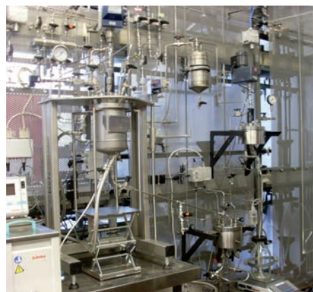
Figure 2: Photography of the miniplant for the continuous production of formic acid.
