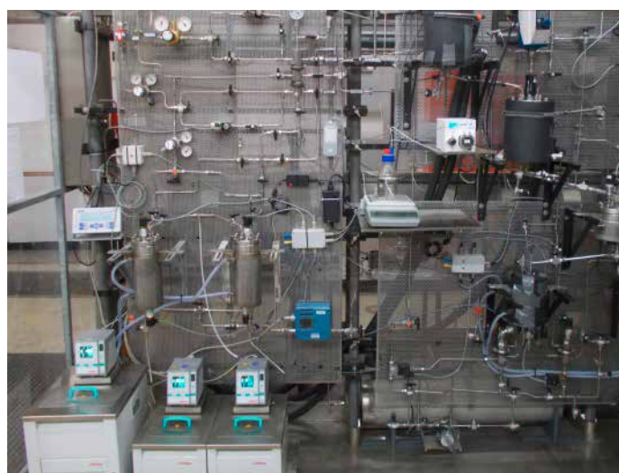
Figure 3: Miniplant for hydroformylation with alternative transition metals
