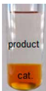
Figure 2: Catalyst recycling via liquid-liquid separation
