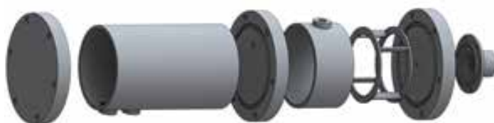
Figure 2. 3D-rendering of finished steel mixer-settler for operation under elevated pressure
