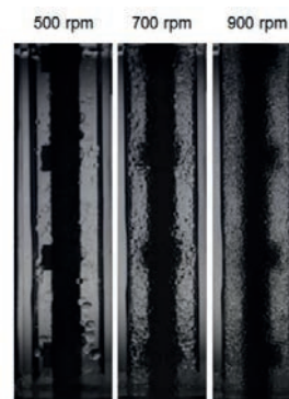
Figure 2: Photos of the dispersion at different stirrer speeds.
