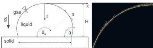
Figure 1: Left-hand side: Draft of the rivulet cross section shape. Right-hand side: Comparison of the rivulet cross section contours under the influence of gravity and with a fixed base width. (---) theoretical results, (—) experimental results, (---) overlapping regions.
