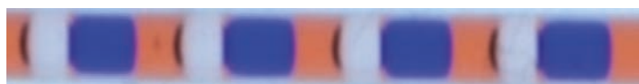
Figure 1: Gas-liquid-liquid triphasic slug flow from right to left in a 1 mm inner diameter capillary. Hexanol (red), Water (blue), Nitrogen (with).
