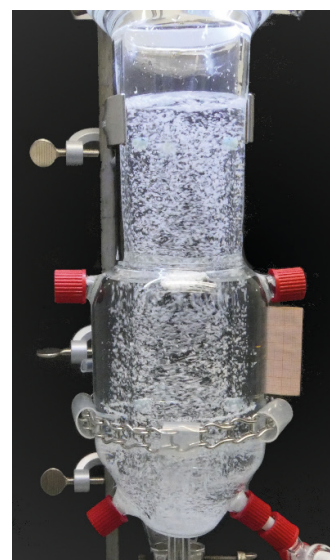
Figure 2: Miniaturized DTB tank during suspension behavior investigations; filled with 1 L suspension and a solid weight fraction of 0.01.
