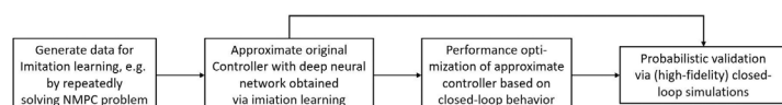
Figure 1: Design process of explicit controllers in the form of deep neural networks.
