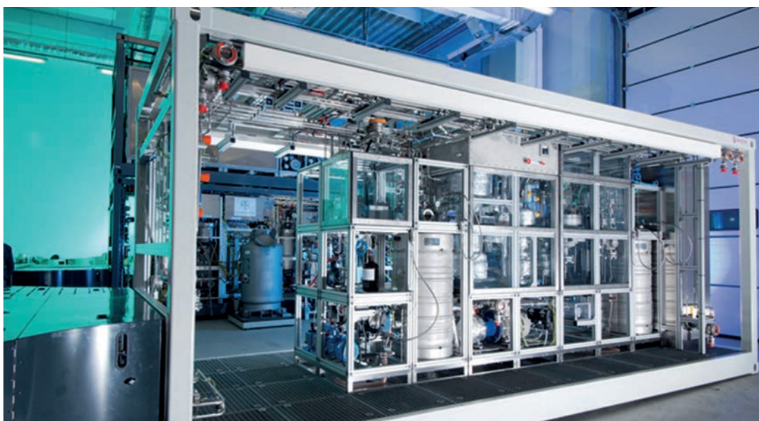
Container setup of modular, small-scale production plant for gas-liquid reactions
