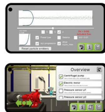
Figure 2. AR-App experiment on turbulent flows and quest system within the pump test rig level.
